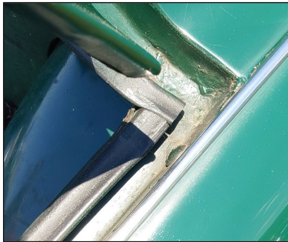
Pre-TS60000 2-piece boot seal joint on RH top of boot opening, the other joint is on LH side.
